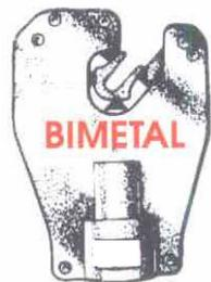
All OPEN THROAT connectors are located in the tool head as shown in the adjacent illustration. The tool nibs are advanced to lightly grip the connector profile at the position where the first crimp is to be made. Subsequent compressions are made by sliding the tool head along the connector.
